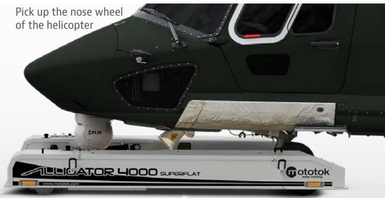
Lifting the nose wheel for manoeuvring
