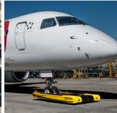
T 7000 Pushback Tug for Aircraft with a MTOW of 75 t
