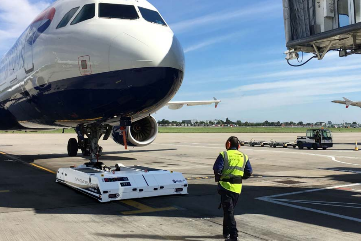
Spacer 8600 NG PB Pushback Tug for Aircraft with a MTOW of 105 t
