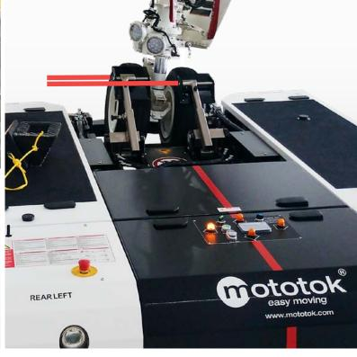
A hydropneumatic system with a nitrogen-filled bladder ensures compensation for double nose wheels
