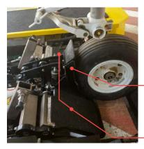
Cage with integrated torque measuring equipment (single wheel)
